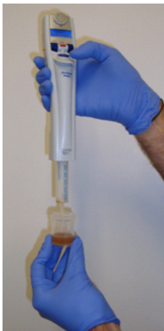
Figure 26 Filling the 10-mL Combipip Plus tip with the aqueous phase and bead mixture using the Xstream pipettor.
