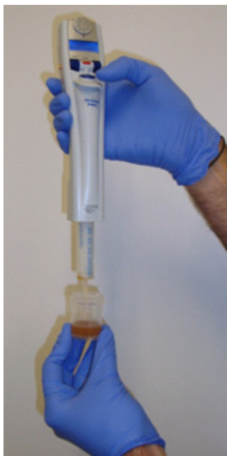
Figure 12 Filling the 10-mL Combipip Plus tip with the aqueous phase and bead mixture using the Xstream pipettor.
