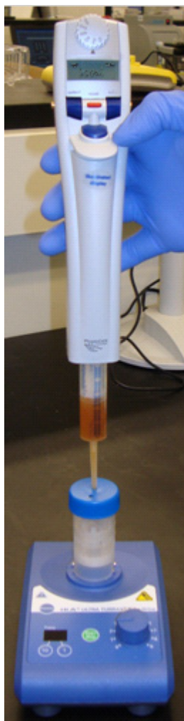
Figure 27 Correct placement of Combitip Plus into sample port in SOLiD™ ePCR Tube cap.
