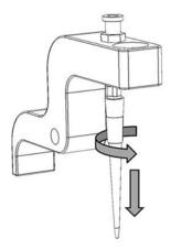
**IMPORTANT!** Improper removal of tips can loosen the metal tip adapter fitting on the Tip Arm and affect instrument operation.
