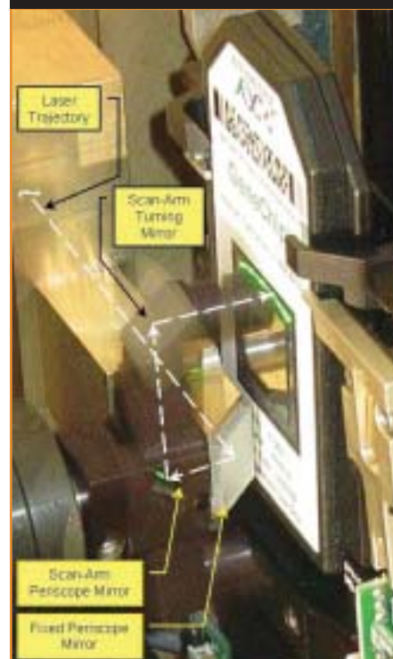
Figure 2: A probe array being scanned by the green laser through the flying objective.
