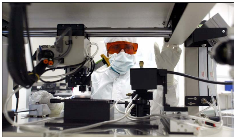
Fig. 16 - Picking and Placing Chips into a Package
