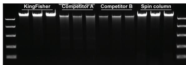
Figure 5. DNA was purified from 1 x 10<sup>6</sup> HeLa-S3 cells with four different competing methods, i.e. the KingFisher Cell and Tissue DNA Kit in conjunction with KingFisher Duo, two competitive magnetic bead systems, and the spin column kit. The KingFisher Cell and Tissue DNA Kit performed very well.
