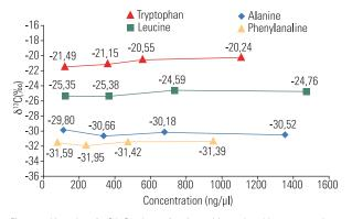
Figure 7: Linearity of <sup>13</sup>C/<sup>12</sup>C values of amino acids analyzed by compound specific isotope analysis *irm*-LC/MS (HPLC mode).
