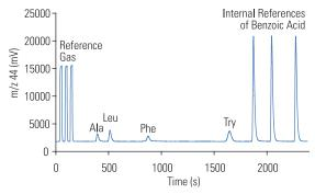
Figure 5: irm-LC/MS chromatogram (m/z 44 trace) of a standard mixture of Ala (113 ng/µl), Leu (123 ng/µl), Phe (79 ng/µl), Try (120 ng/µl).
