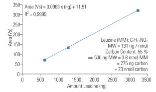
Figure 4: Flow injection irm-LC/MS (µ-EA mode) of leucine, quantitative analysis by correlation of area [in Volt-seconds, Vs] and amount injected [ng].
