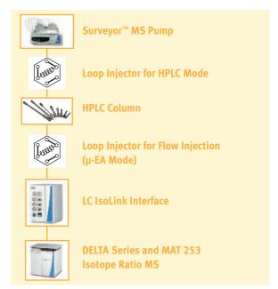
Figure 1: Scheme of the Thermo Scientific  $\it irm$ -LC/MS system with the LC IsoLink.
