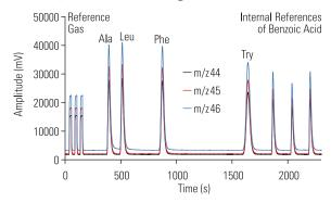
Figure 6: im-LC/MS chromatogram (m/z 44, 45, 46 traces) of a standard mixture of Ala (1354 ng/ $\mu$ l), Lei (1470 ng/ $\mu$ l), Phe (949 ng/ $\mu$ l), Try (1108 ng/ $\mu$ l).
