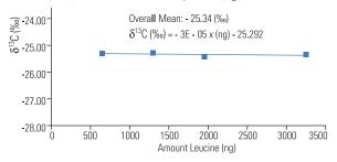
Figure 3: Linearity of leucine analyzed by flow injection  $\it{irm}$ -LC/MS ( $\mu$ -EA mode).
